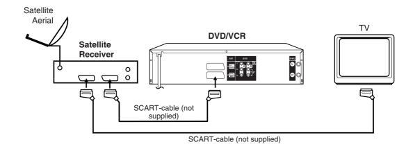
To record from Satellite Receiver press **AUX** on the remote control of DVD/VCR. "L1" will appear on the front display. Select the desired TV-program at Satellite Receiver.
